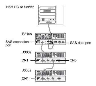
You can expand a SAN system with no single point of failure. See Figure 20. Such an arrangement requires:
